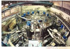
The токамак, a torus-shaped (doughnut-shaped) magnetic chamber<sup>15</sup>, is the most developed magnetic confinement system and is the basis for the design of future fusion reactors using this method. It was invented in the Soviet Union during the 1960s and soon adopted by researchers around the world<sup>16</sup>. The Joint European Torus (JET – pictured), located at Culham Centre for Fusion Energy, is the largest and most powerful tokamak currently operating.
